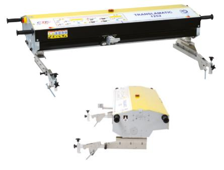
TRANSLAMATIC 1252 robotic arc-welder for positioning the welding gun on the crossing or rail to be repaired with a possibility to move the welding gun up to 1250mm in length (X-axis) and up to 350mm in width (Y-axis).
