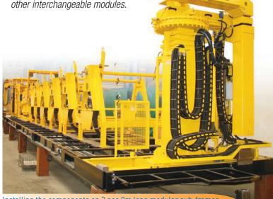
Installing the components on 3 nos 9m long modular sub-frames
