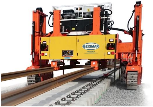
1. ECTR: rail unloading caterpillar gantry
