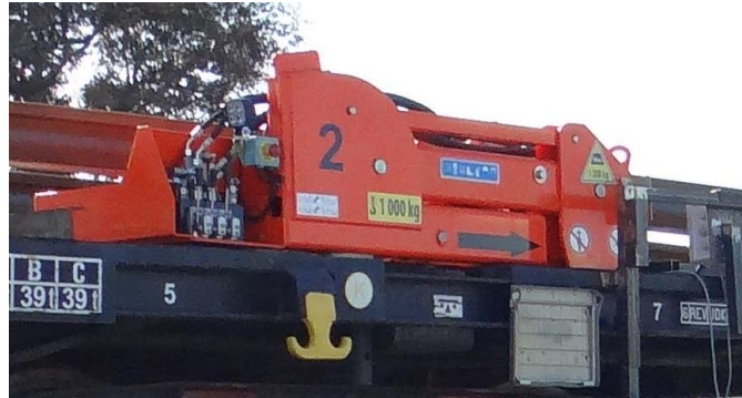
2. RGW: guiding rollers mounted on wagon
