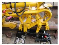
of this machine is that it is possible to extract and insert fastenings simultaneously on each side of the rail.
