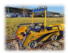
The *VIGILIS 100* can be used to tow or push a *1T* trailer (optional) for the transport of materials and equipment.
