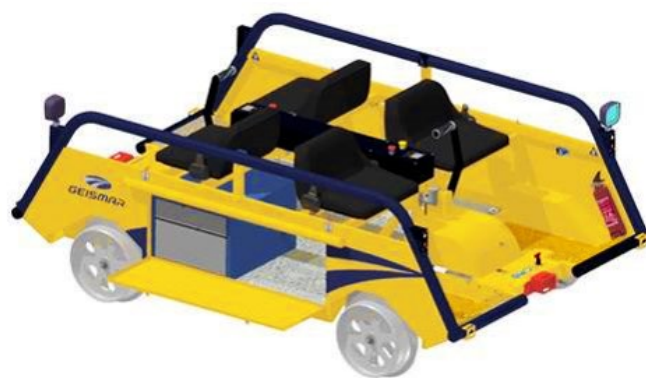
Example of installation of drawers in the chassis of the VIGILIS 100 (up to 4 drawer units)
