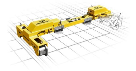
The **Towed Track Recording Unit model EMERALD** is designed to measure track gauge, cross-level, twist and horizontal alignment while being towed behind a road/rail vehicle at speeds up to 20 kph (dependant on the conditions of the track).
